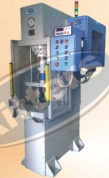
Hydraulic Press 'C' Frame with load cell & safety guard
